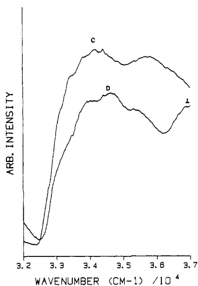
Figure 5. Absorption spectrum of the 32000-37000- \text{cm}^{-1} region of Zeise's salt at 10 K. Band C is the {}^1A_1 \rightarrow {}^1B_2 , xz \rightarrow x^2 - y^2 transition. The remaining transitions are metal to olefin charge-transfer transitions.
